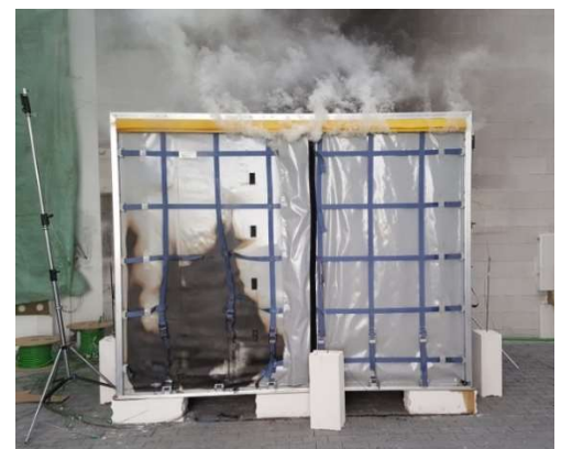
The picture show the successful full scale fire test of an AMJ version of the Nordisk FireShield with net and cover door.
